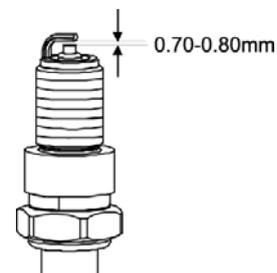
**Note: The engine must be cold**
